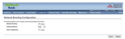
This page is used to configure the network bonding configuration for network interfaces.
