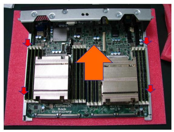
10. Once the edge of black paint touch the chassis iron part, push back the MB self handles back into the self.
