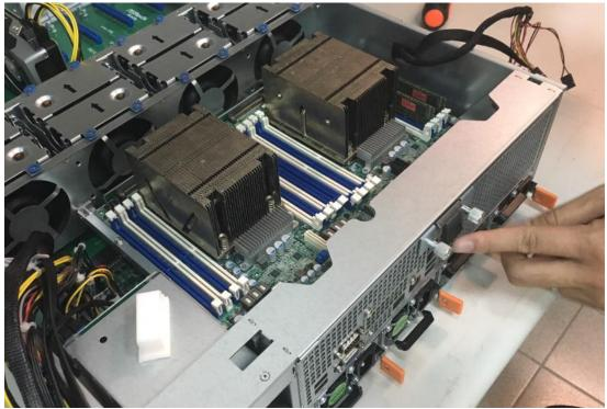
5. Remove 4 screws on side of motherboard tray.
