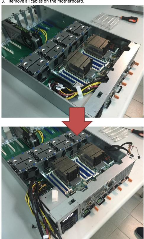
4. Loose front knobs of motherboard tray then push the middle black button to pull tray out.
