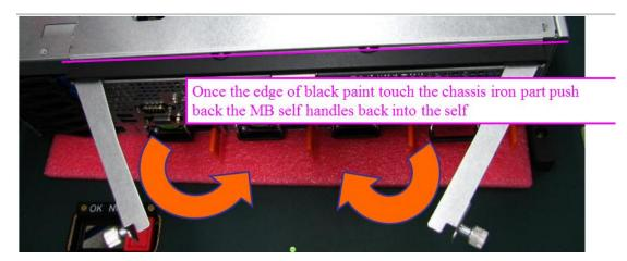
11. Pull out the two handles of MB self and push the MB self by the orange arrow direction into chassis.
